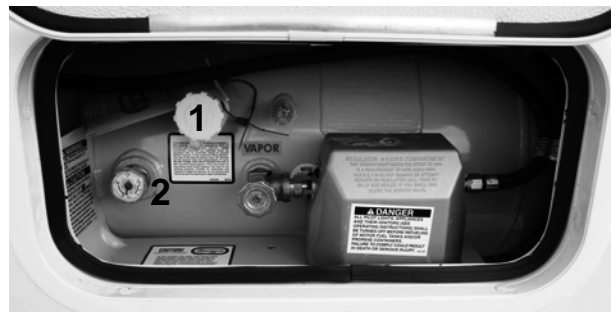
1: Propane fill valve; 2: Propane gauge
